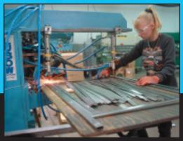
Spot Weld Computerized Control to 200 KVA
